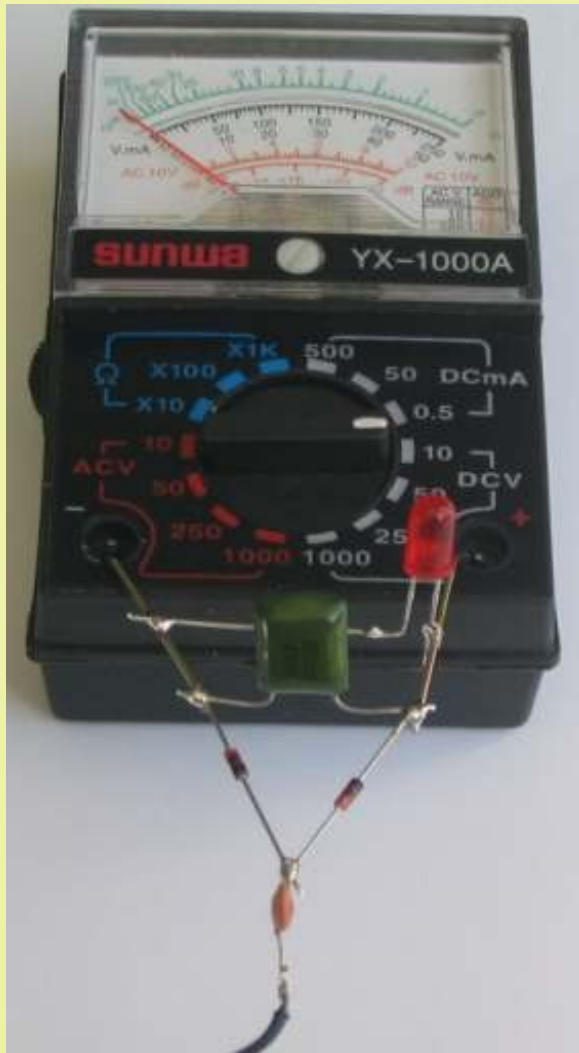
LED Power Meter connected to a
