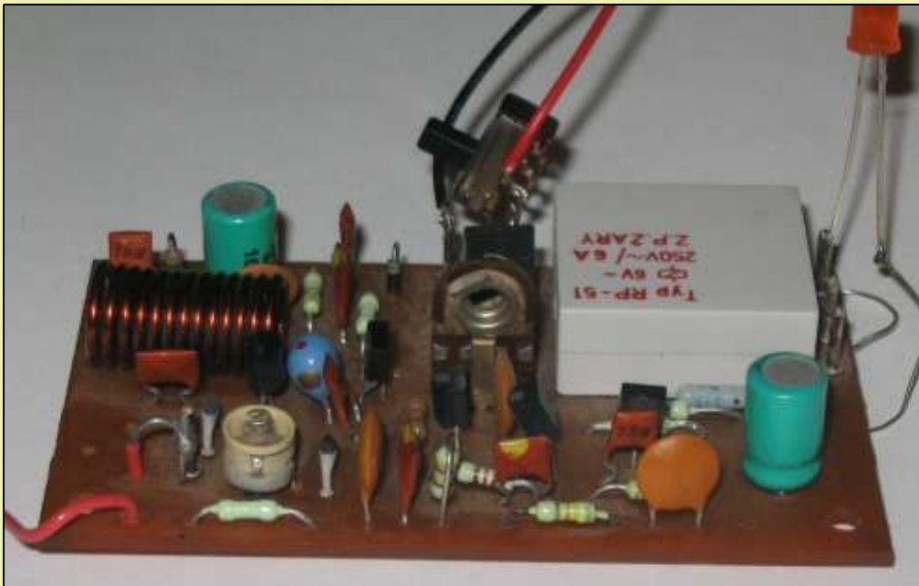
Receiver for transmitter in Circuit B
