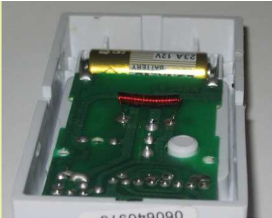
40 turn coil replacing the 1.5uH inductor
