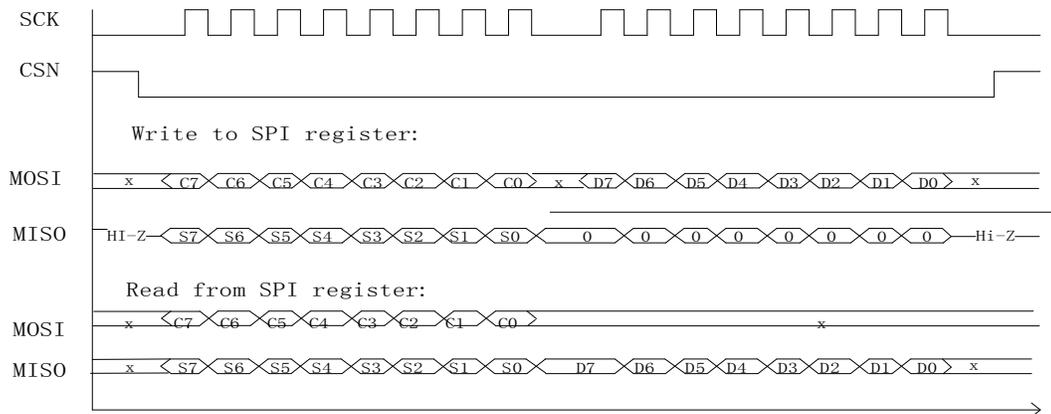
**Figure 6 SPI timing**
