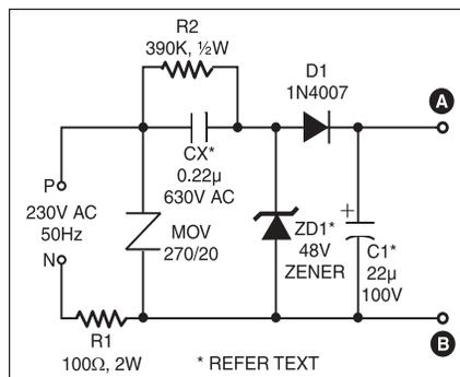
Fig. 1: The circuit of ultra-bright white LED lamp
