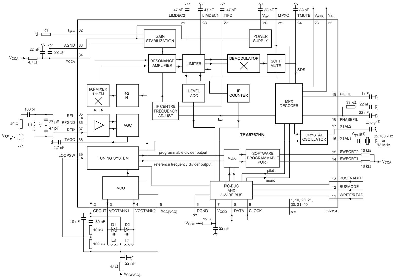
Value of  $C_{pull}$  must be as close as possible to the value of  $C_{load}$  of the crystal.
