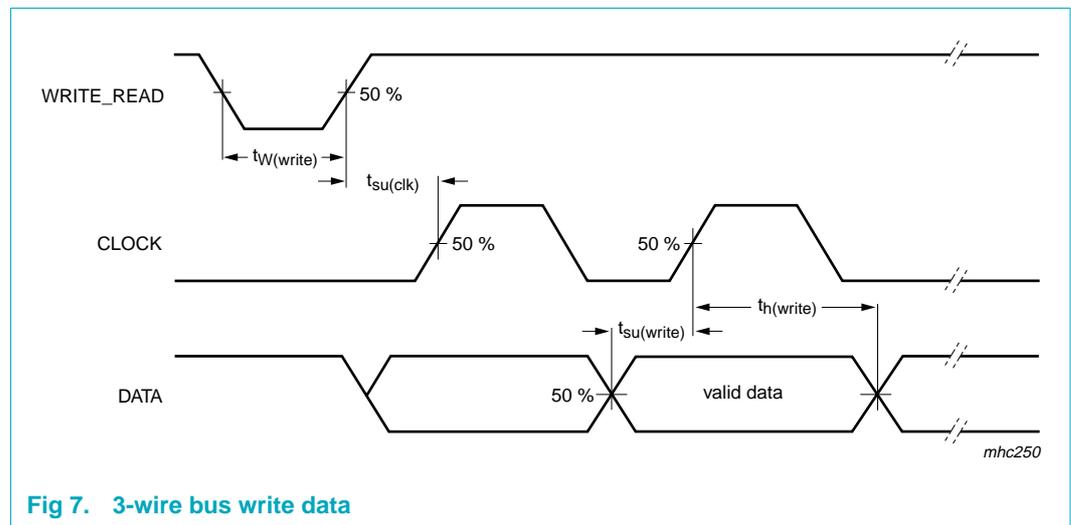
Fig 7. 3-wire bus write data
