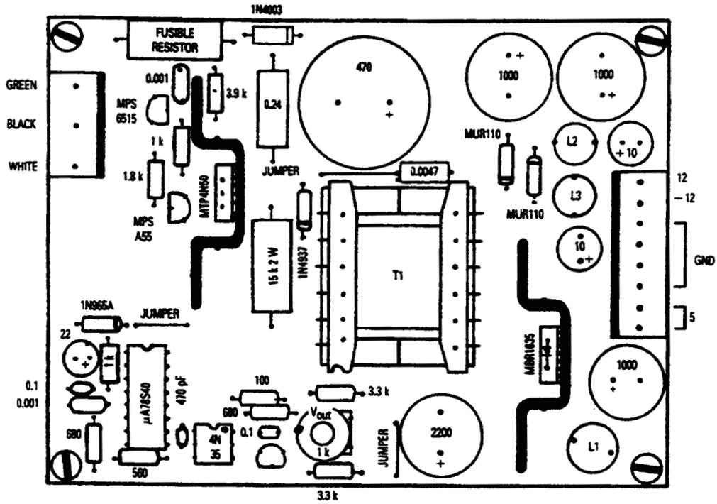
Printed Circuit Board Negative – Bottom View
