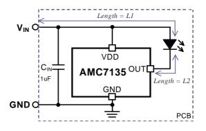
If LED and AMC7135 is located in separate PCBs, or the length of the routing path L1>10cm or L2>3cm, the output capacitor  $C_0$  should be added. Typically, capacitance of  $0.1 \text{uF} \sim 1 \text{uF}$  is recommended and 1 uF is needed when L2 is much longer than 3cm.
