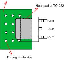
Recommended figure of PCB area used as a heat sink.
