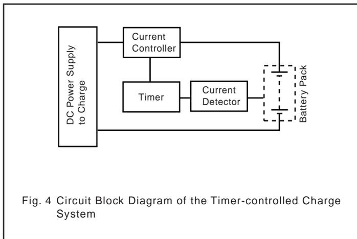
Fig. 4 Circuit Block Diagram of the Timer-controlled Charge System
