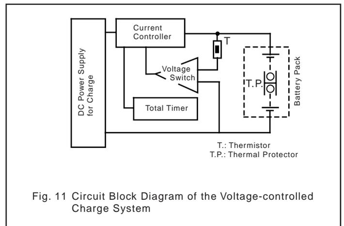
Fig. 11 Circuit Block Diagram of the Voltage-controlled Charge System
