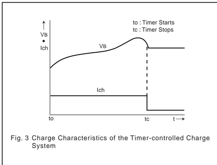
Fig. 3 Charge Characteristics of the Timer-controlled Charge System
