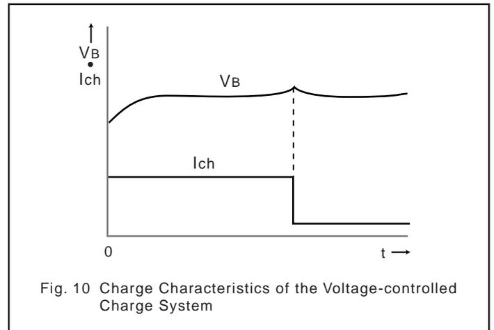
Fig. 10 Charge Characteristics of the Voltage-controlled Charge System
