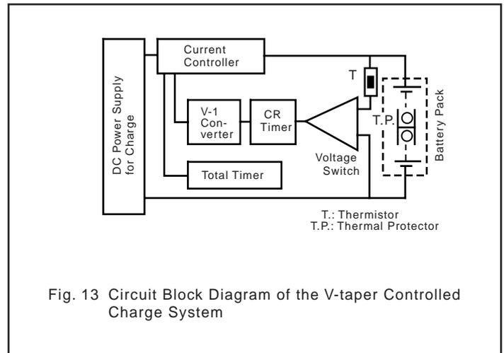
Fig. 13 Circuit Block Diagram of the V-taper Controlled Charge System
