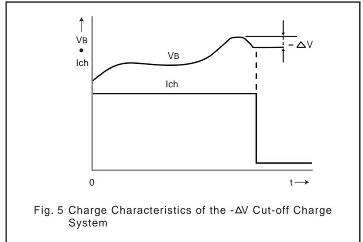
Fig. 5 Charge Characteristics of the  $-\Delta V$  Cut-off Charge System
