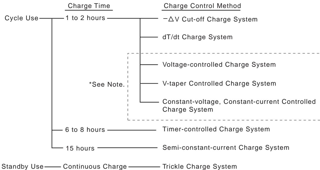
\* Not a recommended charge method for Ni-Cd batteries
