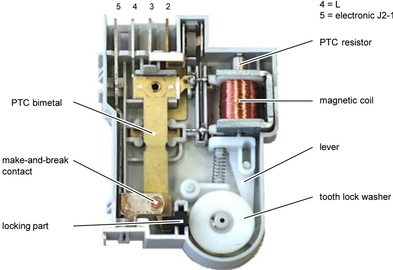
**When closing** the lid the door lock gets an impulse from the electronic by contact 3. The impulse feeds the magnetic coil over the PTC resistor. This moves the lever down and the tooth lock washer is forwarded by another tooth. This can be heard by a click. The locking part is unlocked, the lid is closed.
