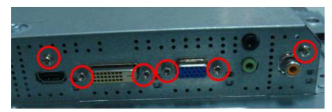
2. Release 3 screws on MAIN BOARD.
