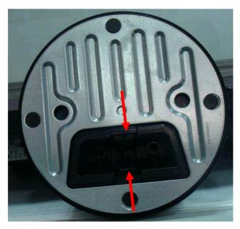
2. Use C/D disassembly tool to unlock STAND COVER.
