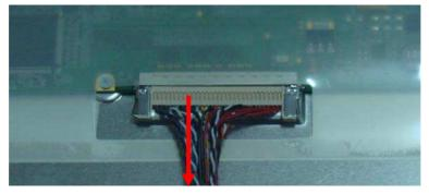
4. Remove the MAIN SHIELDING away from the LCD PANEL.
