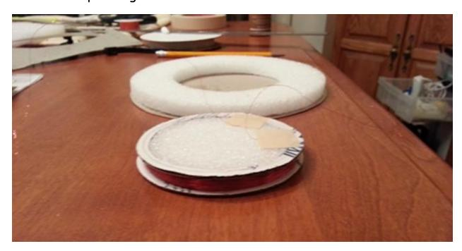
The Tx coil is made on a separate former and held together with Cyan glue. Then this coil is simply glued into a channel cut into the foam.
