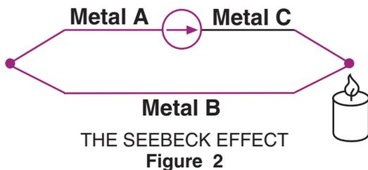
If this circuit is broken at the center, the net open circuit voltage (the Seebeck voltage) is a function of the junction temperature and the composition of the two metals.
