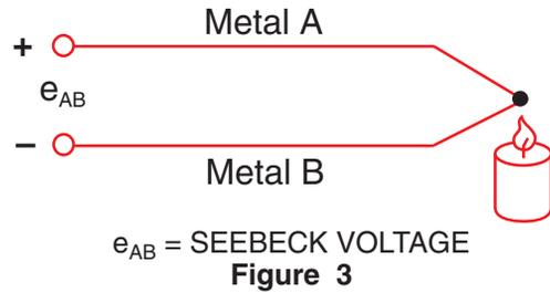
All dissimilar metals exhibit this effect. The most common combinations of two metals are listed in **Appendix B** of this application note, along with their important characteristics. For small changes in temperature the Seebeck voltage is linearly proportional to temperature:
