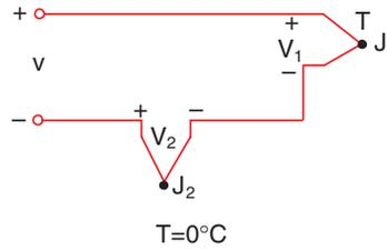
The copper-constantan thermocouple shown in Figure 5 is a unique example because the copper wire is the same metal as the voltmeter terminals. Let's use an iron-constantan (Type J) thermocouple instead of the copper-constantan. The iron wire (Figure 6) increases the number of dissimilar metal junctions in the circuit, as both voltmeter terminals become Cu-Fe thermocouple junctions.
