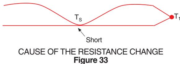
The new junction will measure temperature  $T_s$ , not  $T_1$ . The resistance measurement has given us additional information to help interpret the physical phenomenon detected by a standard *open thermocouple* check.
