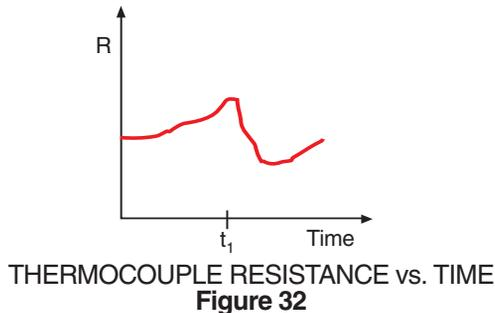
The resistance of a thermocouple will naturally change with time as the resistivity of the wire changes due to varying temperature. But a sudden change in resistance is an indication that something is wrong. In this case, the resistance has dropped abruptly, indicating that the insulation has failed, effectively shortening the thermocouple loop.
