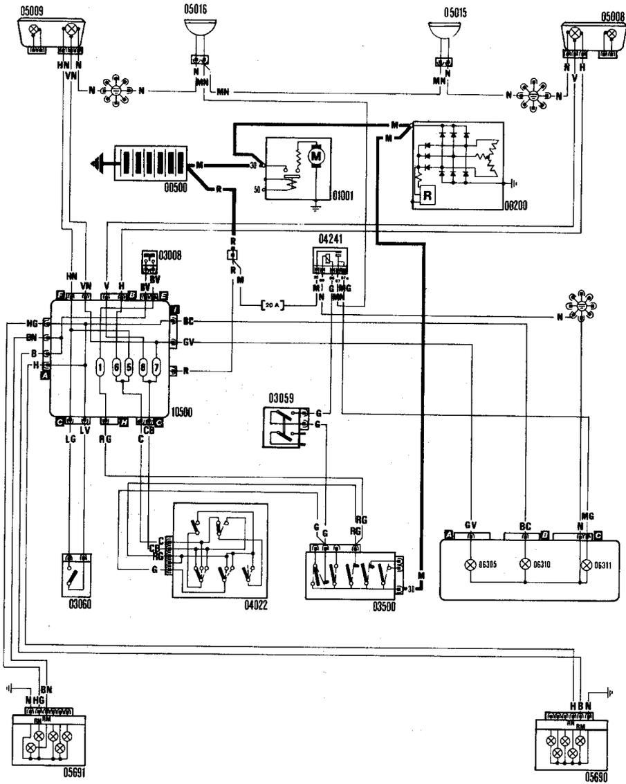
Wiring diagram 7. headlamps, reversing lamps and front and rear foglamps
