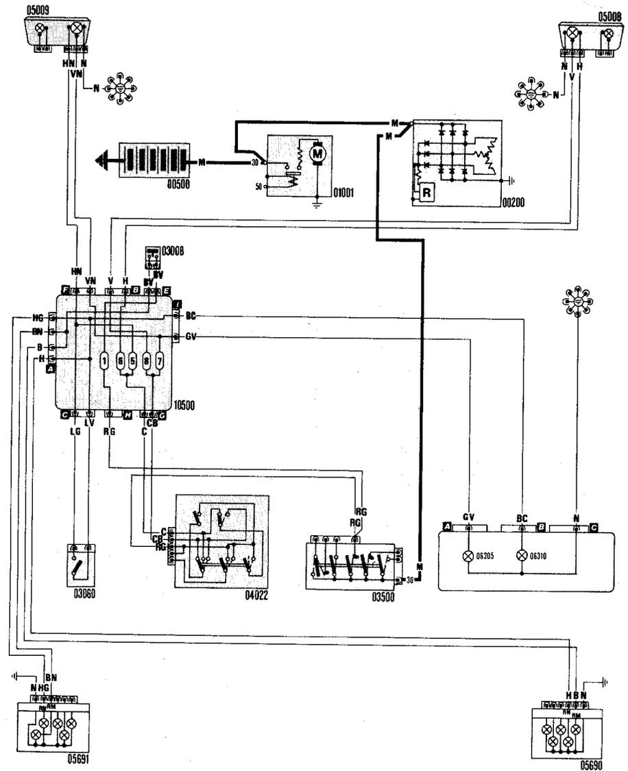
Wiring diagram 8. headlamps, reversing lamps and rear foglamps (Comfort)
