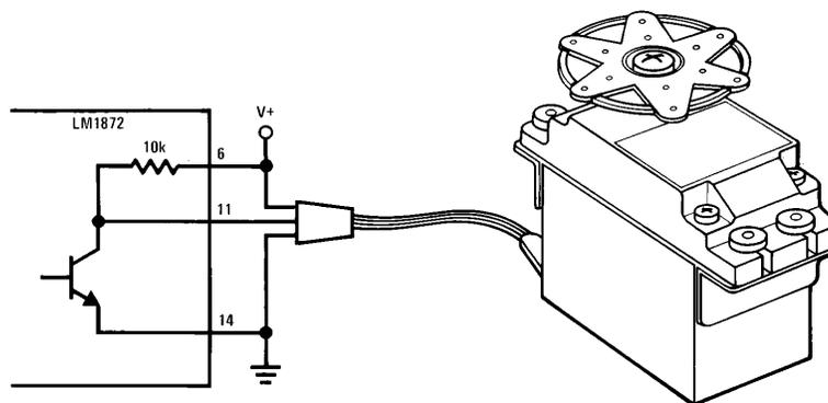
FIGURE 15. Interfacing Directly to Standard Hobby Servos
