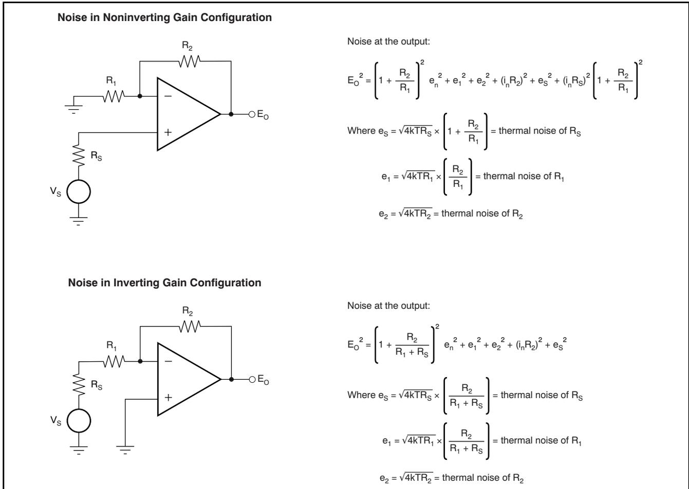
For the OPA161x series op amps at 1kHz,  $e_n = 1.1\text{nV}/\sqrt{\text{Hz}}$  and  $i_n = 1.7\text{pA}/\sqrt{\text{Hz}}$ .
