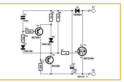
Figure 1. The circuit is designed to employ a kind of bootstrapping effect when the FET gate is driven.
