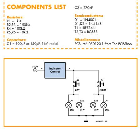
Figure 3. Connection diagram of the turn indicator incorporating the all-solid state drive circuit.
