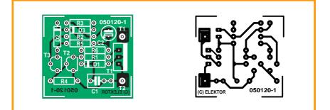
Figure 2. The circuit board is so small it can usually be fitted into the original turn indicator control box.
