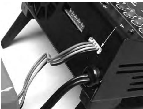
Please check the polarity of the battery carefully: the black wire must be connected to the pin marked with an arrowhead printed on the case.
