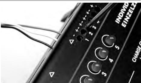
The Lipomat battery charger features a second, alternative socket for Voltage Sensor leads which do not conform to the robbe norm. The user's own connector system can be connected to the charger using the screw terminals. The battery must be wired in the same manner. The common negative terminal (black wire) must be connected to terminal 1, which is marked with an arrowhead.
