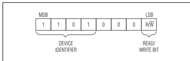
Figure 8. I<sup>2</sup>C Slave Address Byte
