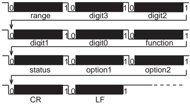
The meter always outputs the current input value to the serial port regardless of whether the hold function has been activated or not. Each block is repeated twice in one conversion cycle. The detailed data format of each packet is listed below.
