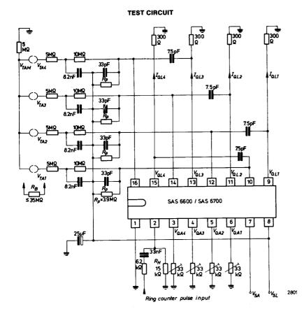
NOTE Supply voltage must be disconnected before inserting the integrated circuit in the socket.
