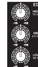
Fig. 2.5: The equalizer of the stereo input channels
