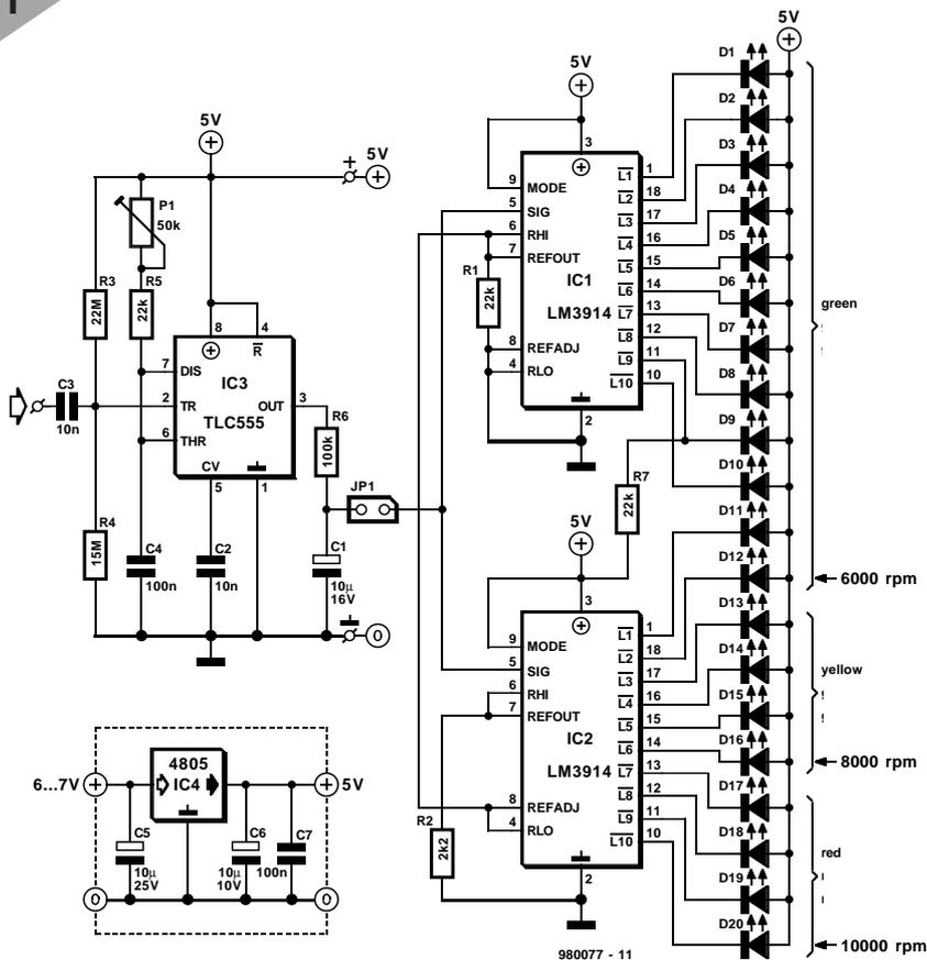
**Figure 1.** The circuit of the tachometer consists of a pulse shaper, an integrating circuit, and a readout. The sensor is placed around the spark plug cable.
