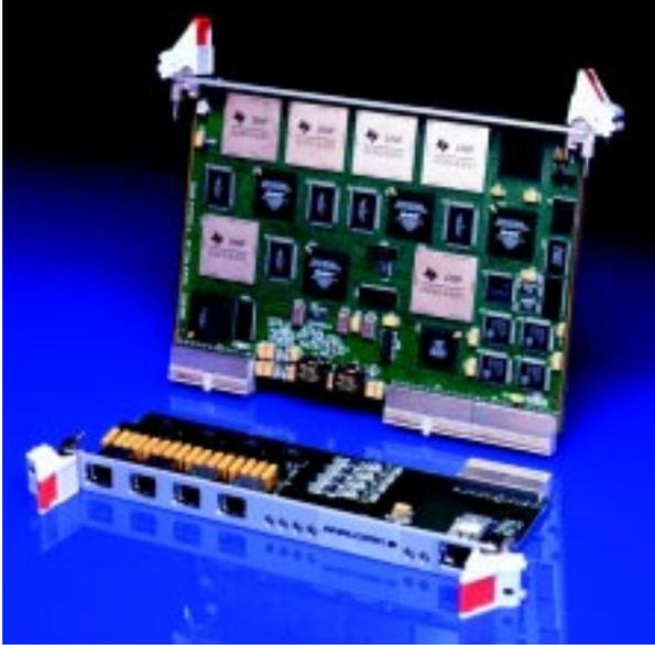
This card lets voice and data entering the T1/E1 interface be compressed by the DSP resource and exit through the Ethernet interface without unnecessary processing by the host or bandwidth transfers over the bus. The host is free to manage call setup and teardown and to calculate and support custom calling features for packet-switched calls.
