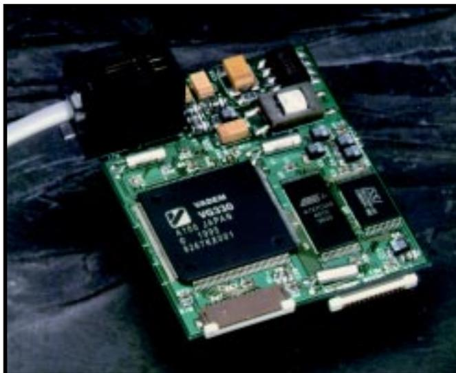
Photo 1—The Vadem IPump reference design uses their VG330 PC-on-a-chip to enable EPCs to get a piece of the Internet-appliance action.
