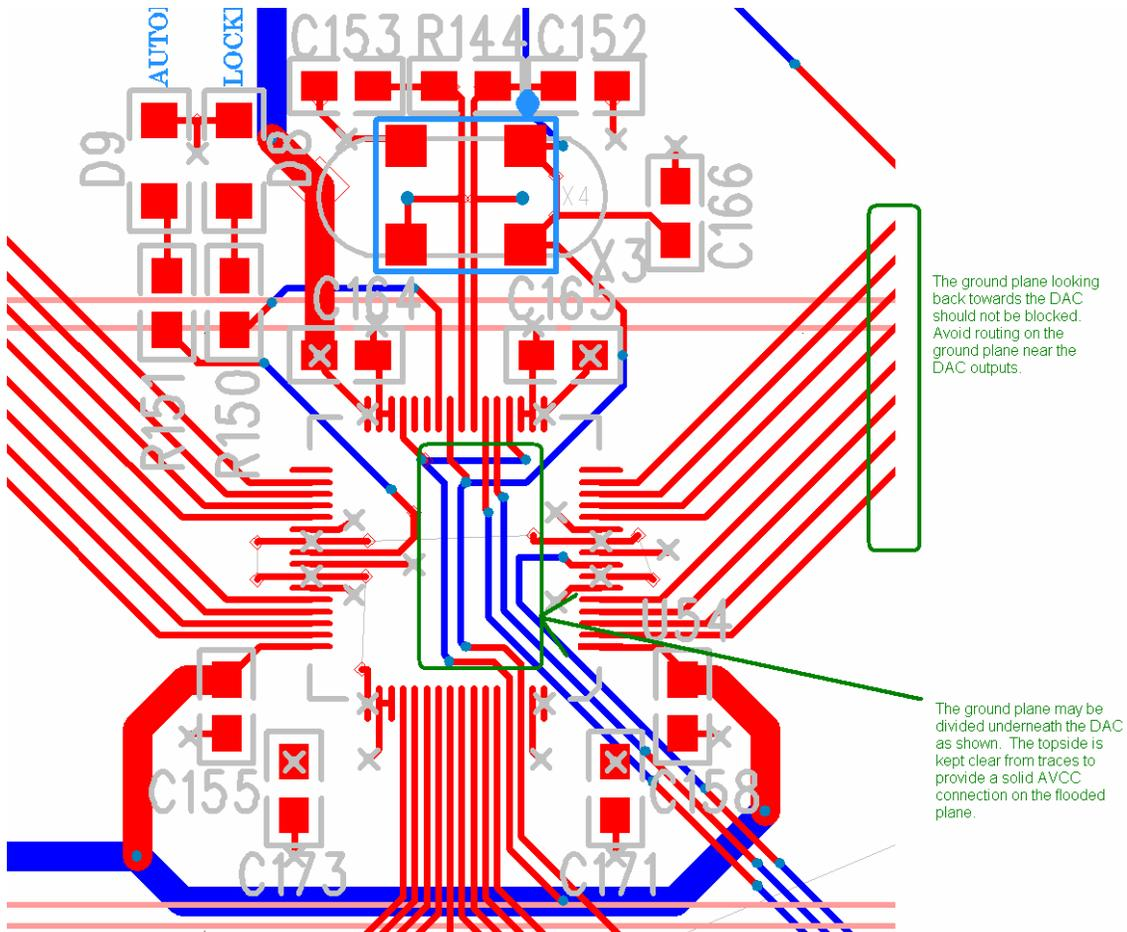
The ground plane looking back towards the DAC should not be blocked. Avoid routing on the ground plane near the DAC outputs.
