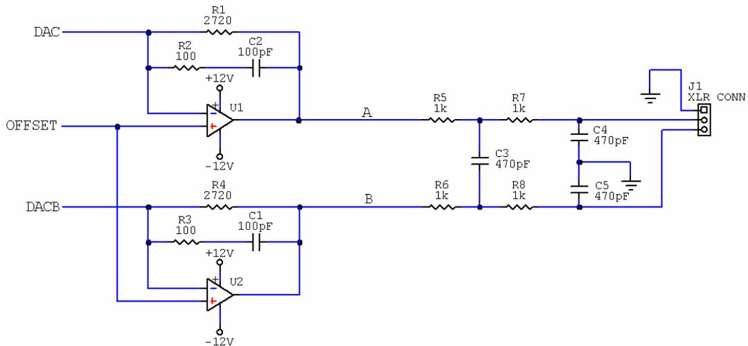
**Figure 1: Sabre Reference Evaluation Board Differential Output**
