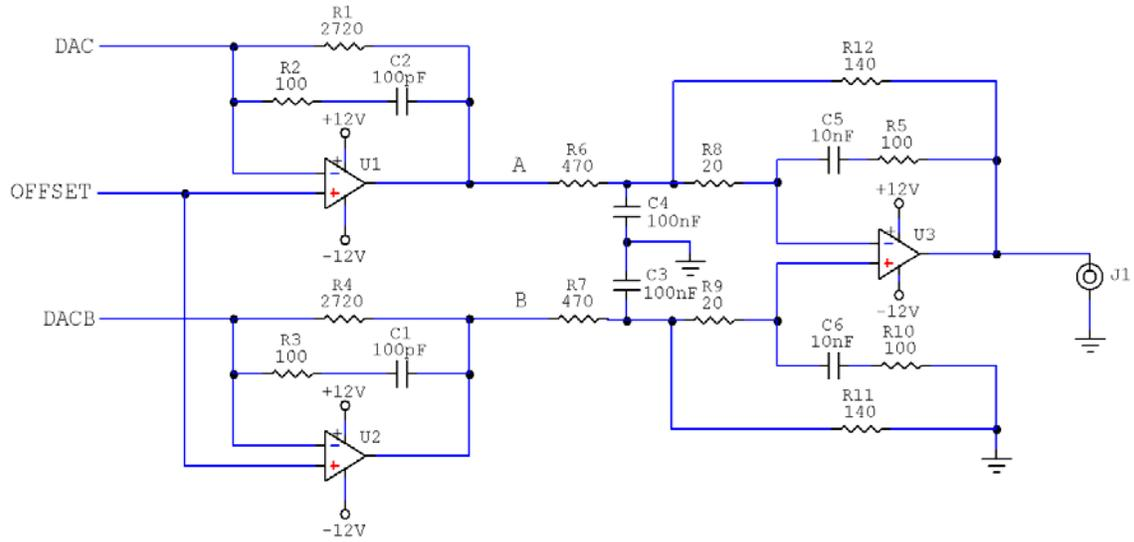
**Figure 2: Sabre Reference Evaluation Board Single Ended Output**
