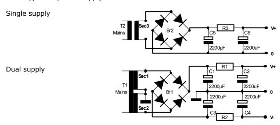
Whereas the filtering resistors R1, R2 and R3 may serve as dropper resistors, instead of the resistors placed at the shunts themselves, and are calculated the same way. We recommend Schottky diodes for B1 and B2.
