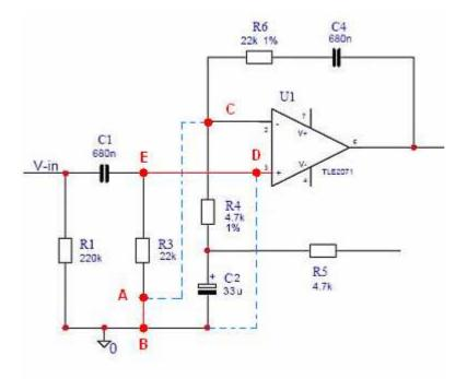
The input-cap is connected directly to the positive input (E-D) and the input-high-pass (C1, R3) is passive now (A-B). The former (blue) connections (A-C, D-B) are eliminated. Some components have to be changed as well:
