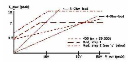
In any case, there probably will not be THD  $\leq$  0.01% at all 'unprotected' levels after this mod, for sure, and not 50W \_continuous\_ sine-drive into 2 Ohm (so you have to take some care not to overheat the amp when driving low-impedance-loads with continuous signals on the workbench!) -- but there will be no interference by the protection-circuit during for example 7A-peaks into 2 Ohm ( $\sim$ 50W).
