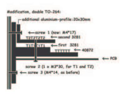
Mount the 3281s (resp. their successors) close to the 40872-side to leave enough room for screw\_1. Place the lower two (Tr1) first, then add the profile with screw\_1, then the upper two (Tr2) and at last screw\_2 (the nut on top of TR2). All transistor-packages must be insulated with suitable pads and heat-transfer-compound has to be used. To my experience the cooling of all four devices is excellent then.
