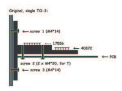
The second pair can conveniently be mounted on top of the first. To insure proper cooling, add a small aluminium-profile (2cm+3cm, ~8cm long, 3mm or 4mm; with 4 suitable 4.5mm-holes for the screws):
