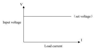
In other load modes, press 【V-SET】 key to enter constant voltage mode. Press 【ON/OFF】 key to start or stop working.
