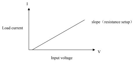
In other load modes, press [R-SET] key to enter constant resistance mode. Press [ON/OFF] key to start or stop working.
