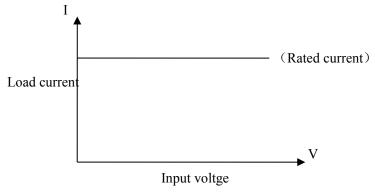
In other load modes, press [I-SET] key to enter constant current mode. Press [ON/OFF] key to start or stop working.
