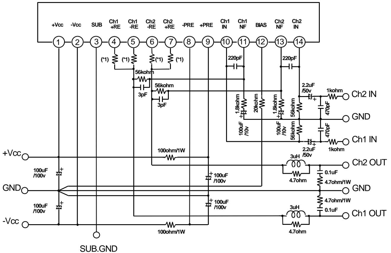
(\*1)Metal Plate Cement Resistor 0.22ohm+-10%(5W)
