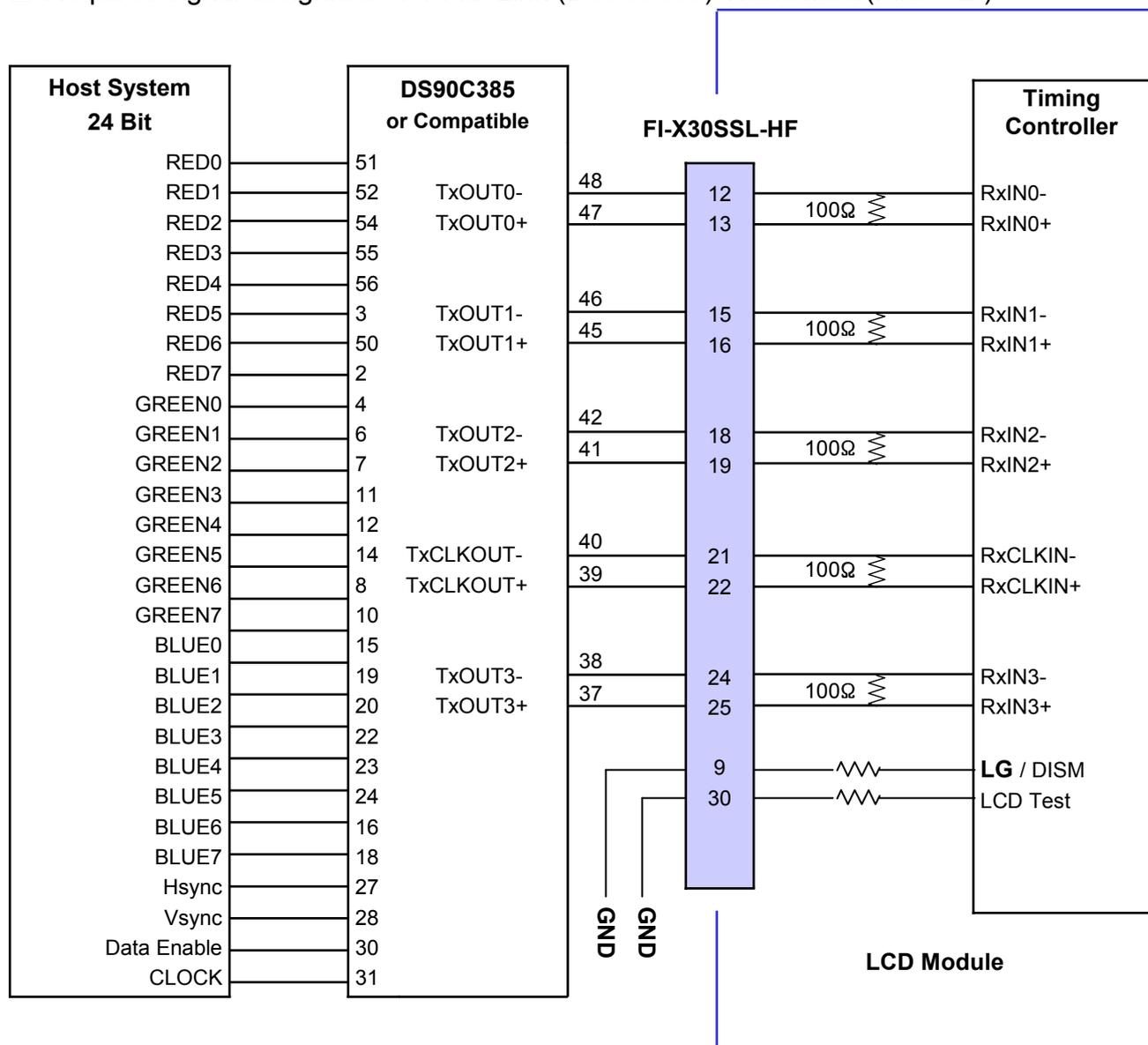
Note: 1. The LCD Module uses a 100 Ohm[Ω] resistor between positive and negative lines of each receiver input.
