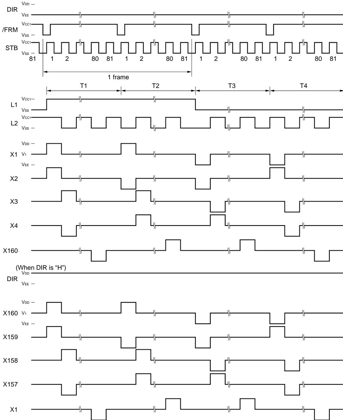
**Remark** When /DOFF' is "L", the X output becomes V<sub>1</sub> level. Afterward, if /DOFF' becomes "H", the level of the X output is output with the above timing.
