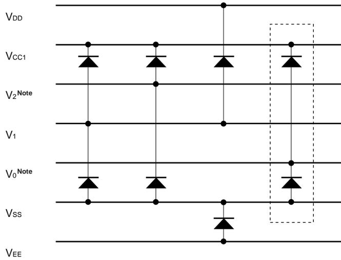
Connect the diodes enclosed in the dotted line ( [ ] ) when  $V_0$  is not 0 V (GND)
