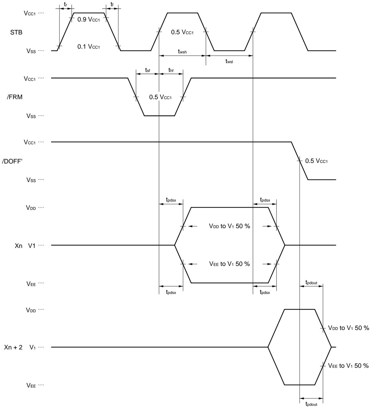
**LEVEL SELECTION TIMING OF LIQUID-CRYSTAL DRIVE OUTPUT**
