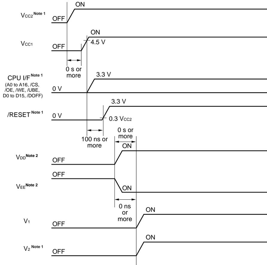
**Notes** 1.  $V_{CC2}$ , CPU I/F,  $\text{/RESET}$ , and  $V_2$  are column driver power supply pins or input pins.
