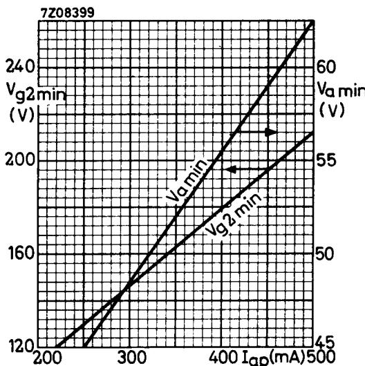
Minimum required values of the screen grid voltage and of the anode voltage when the tube is used in line output stages. The graphs refer to nominal mains voltage provided the specified values of  $V_a$  are increased by 10% of the anode supply voltage. The specified values of  $I_{ap}$  will be available throughout life of the tube at supply voltage values 10% below nominal.
