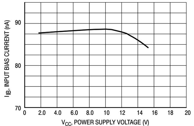
Figure 9. Input Bias Current versus Power Supply Voltage
