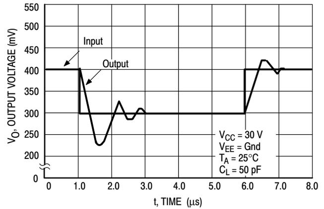
Figure 7. Small-Signal Voltage Follower Pulse Response (Noninverting)
