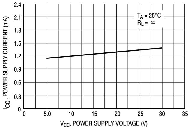
Figure 8. Power Supply Current versus Power Supply Voltage
