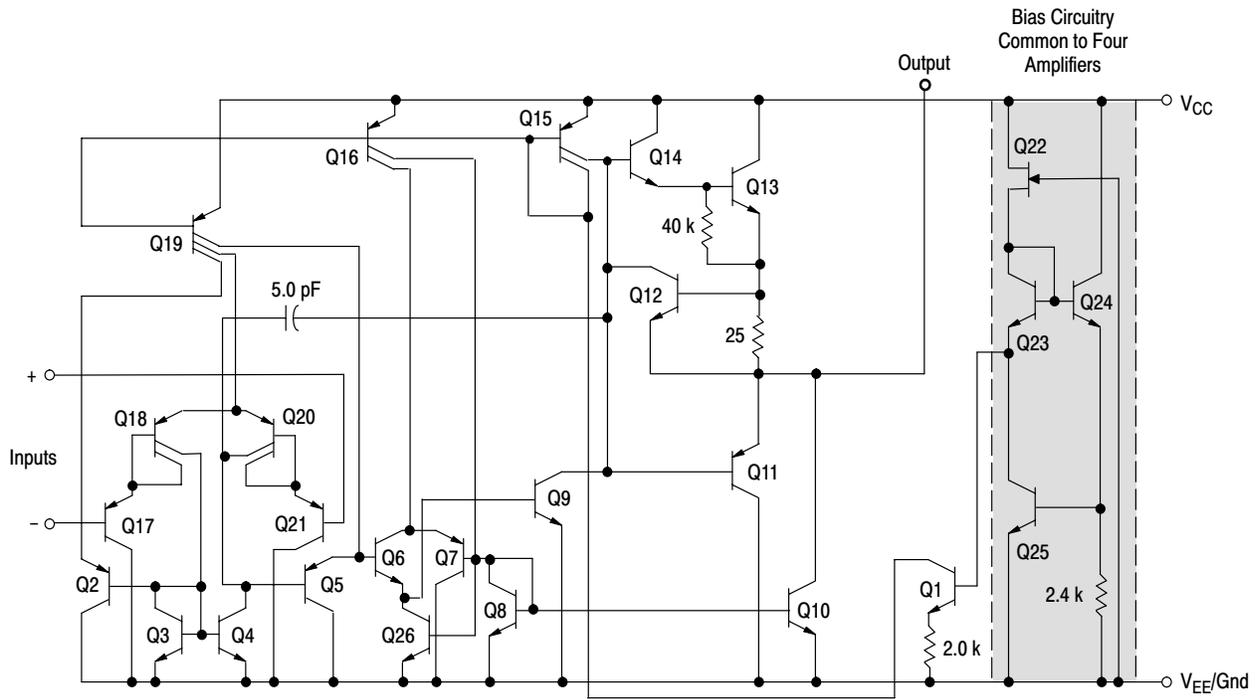
Figure 1. Representative Circuit Diagram
