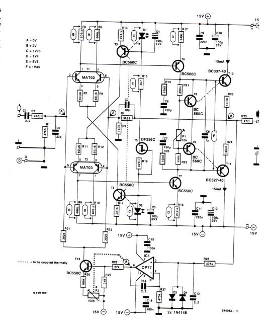
Fig. 1. Circuit diagram of the discrete preamplifier
