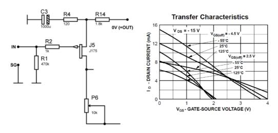
20 mA. From the characteristic below you can see that our 1.8kohm resistor ( $R_{14}$ ) will give about  $I_D$  = 1.5 mA of drain current for VGS = 2.7 V as the quiescent point for  $J_5$  (assuming that the output is at 0V DC), since  $I_D = V_{GS}/R_{14}$ . The potentiometer  $P_6$  is used to set the working point for  $M_{18}$  (and  $M_{11}$ ). The gain in the first stage is given by the transconductance of the JFET and the resistors  $R_4$
