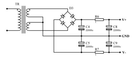
However, this was not sufficient for the negative leg ( $M_{11}$  and  $M_{18}$  is operating in common gate for signals on the negative leg), causing a ripple at the amplifier output that was annoying. So one more RC section was added at the negative rail with another one ohm resistor and 22000  $\mu$ f capacitor. A better solution would probably be to use a capacitance multiplier instead of all the RC-filtering.
