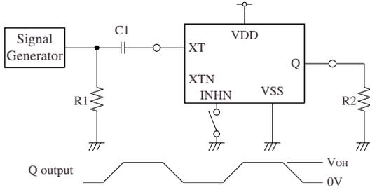
1.0V<sub>p-p</sub>, 10MHz sine wave input signal
