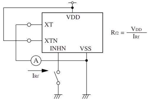
$$R_{f2} = \frac{V_{DD}}{I_{rf}}$$
