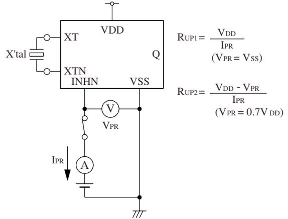
$$R_{UP1} = \frac{V_{DD}}{I_{PR}} \quad (V_{PR} = V_{SS})$$
