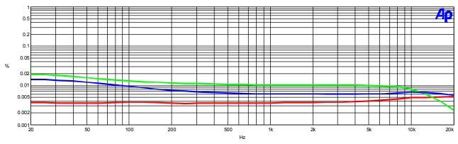
From top to bottom: 40W, 10W, 1WFrequency Response ( $4\Omega$ ,  $8\Omega$  and open circuit)
