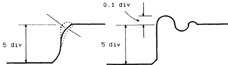
[21] Check/Adjust Attenuation Compensation ( ATT  $\div 10$ ,  $\div 100$  ).
