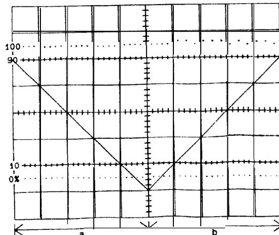
\* Adjust the length of a & b may be equal (in the time axis).
