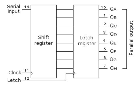
An outline of the 74HC595 shift register connections is shown on the diagram below:
