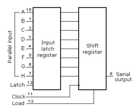
An outline of the connection of the shift register 74HC597 to a micro, is shown below.
