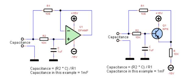
Left figure above : R2 and C form an integrator. The OPAMP U1 is configured as a voltage follower, so the capacitor voltage at the non-inverting input also appears on the non-inverting input. This means that the voltage over R1 is equal to the voltage over R2. But because R1 is 1000 times lower than R2, R1 will draw extra current
