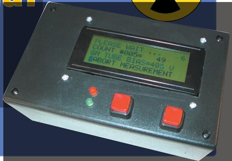
**There is something fascinating about an instrument that can sense that which is invisible and undetectable to all human senses. This article is about the design and building of a portable Digital Geiger Counter (DGC) device as shown in the photos with many unique features**
