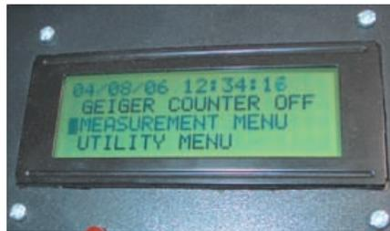
Fig.6: The LCD display after welcome on power-up
