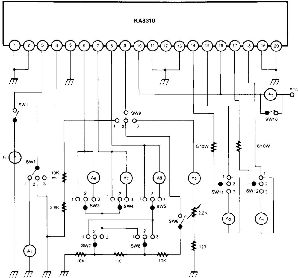
TEST METHOD ( $V_{CC}=12V$ )
