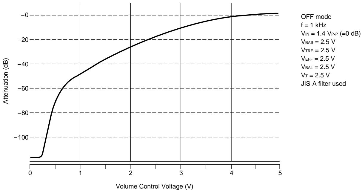
**Remark** L<sub>L+R</sub>: L+R volume control voltage, V<sub>BAS</sub>: Bass control voltage,
