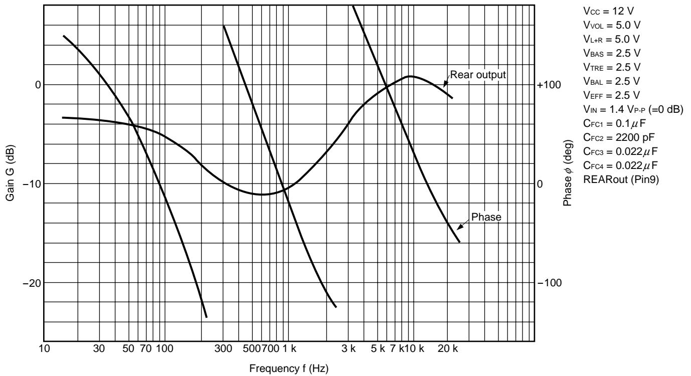
**Remark**  $V_{VOL}$ : Volume control voltage,  $V_{L+R}$ : L+R volume control voltage,  $V_{BAS}$ : Bass control voltage,  $V_{TRE}$ : Treble control voltage,  $V_{BAL}$ : Balance control voltage,  $V_{EFF}$ : Effect control voltage,  $C_{FC1}$ ,  $C_{FC2}$ ,  $C_{FC3}$ ,  $C_{FC4}$ : External capacitance connected to FC1 to FC4 (Pin 2 to 5).
