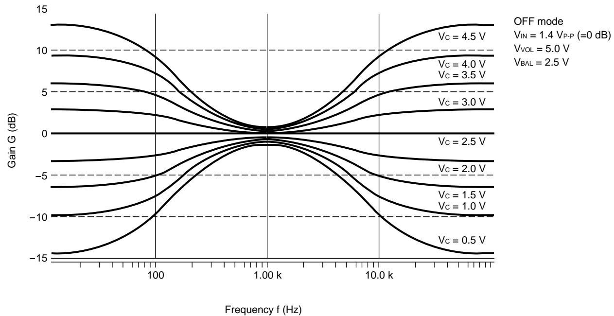
**Remark**  $V_{BAL}$ : Balance control voltage,  $V_{VOL}$ : Volume control voltage,  $V_c$ : Bass, Treble control voltage.
