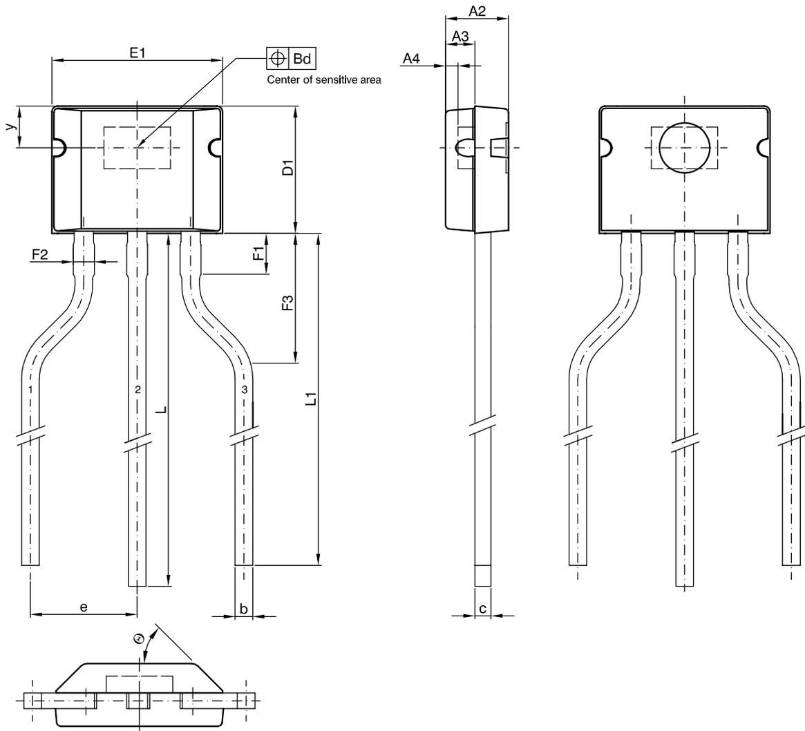
solderability is guaranteed between end of pin and distance F1.
