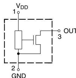
**Fig. 1–1:** Pin configuration
