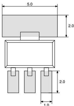
**Fig. 3–6:** Recommended pad size SOT89B-1
