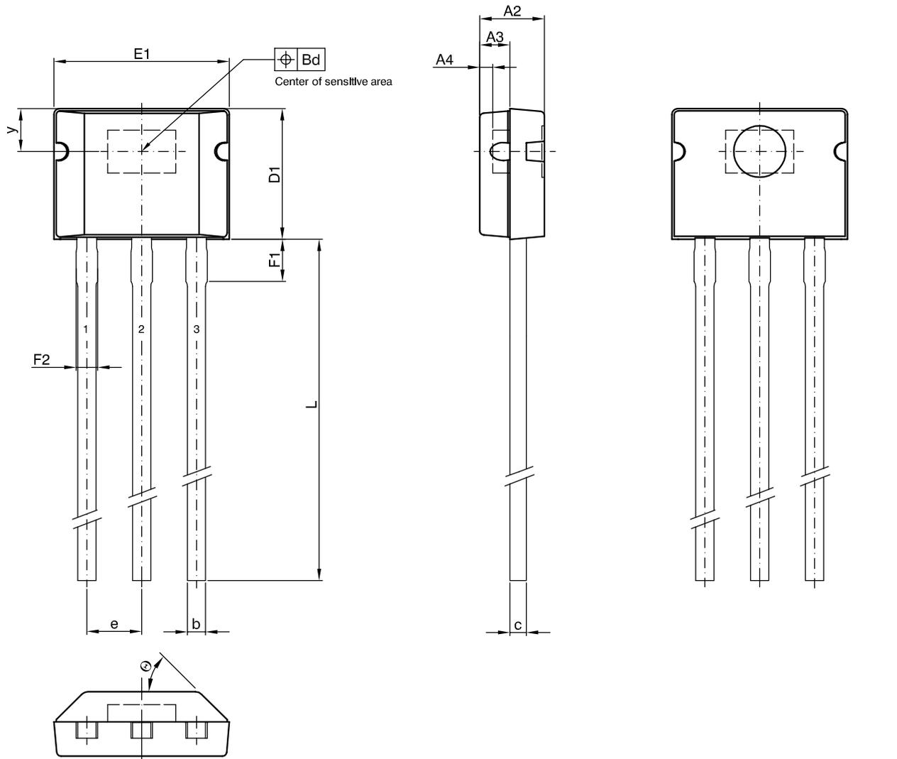
solderability is guaranteed between end of pin and distance F1.
