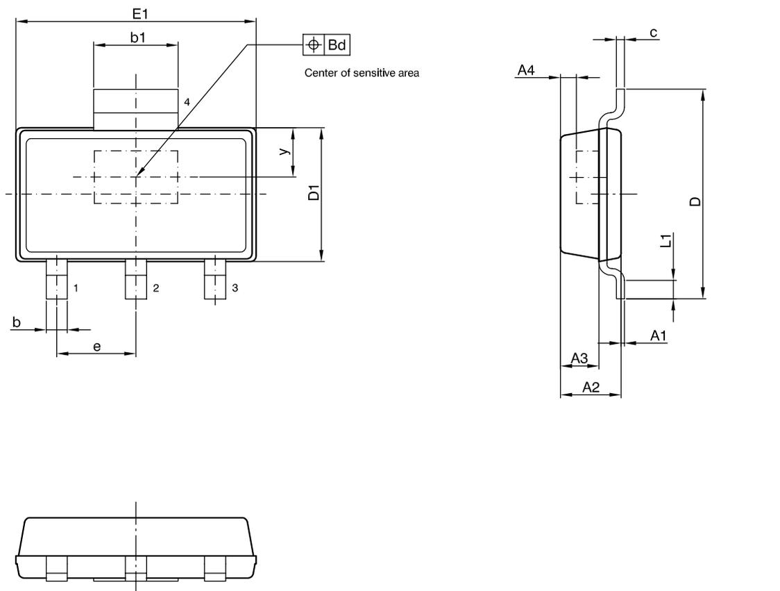
y= this dimension is different for each sensor type and is specified in the data sheet.
