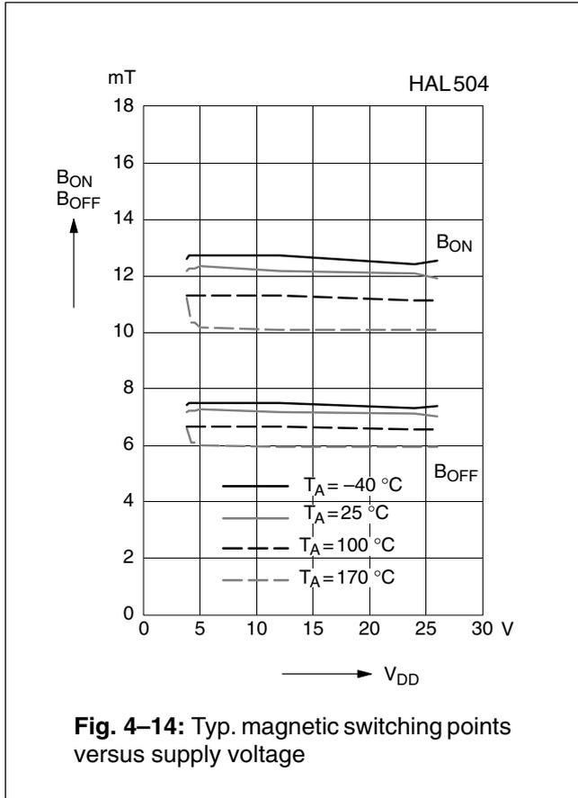
**Fig. 4-14:** Typ. magnetic switching points versus supply voltage
