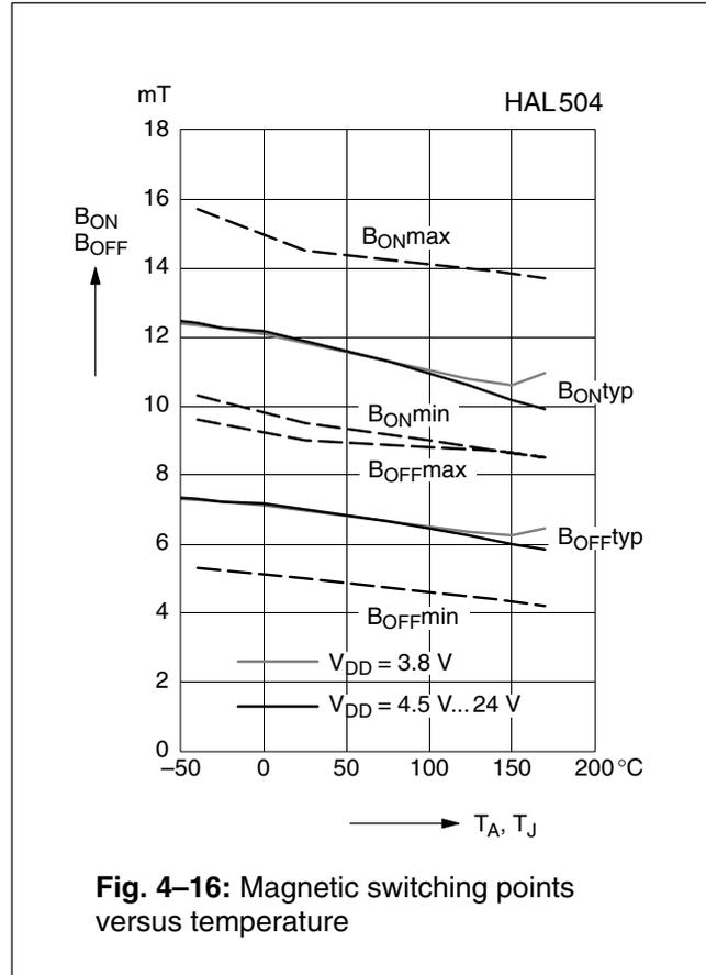
**Fig. 4-16:** Magnetic switching points versus temperature
