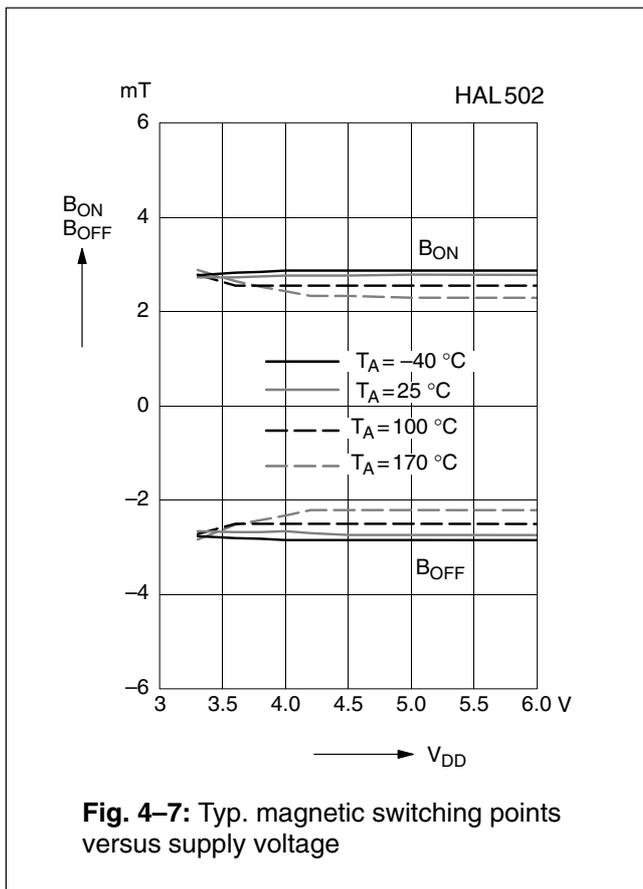
**Fig. 4-7:** Typ. magnetic switching points versus supply voltage
