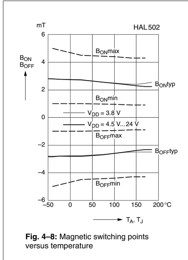
**Fig. 4-8:** Magnetic switching points versus temperature
