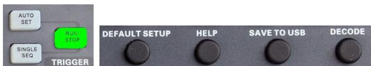
**Auto Set:** Automatically set the oscilloscope controls to generate a usable display of the input signals. Refer to the following table for relative content.
