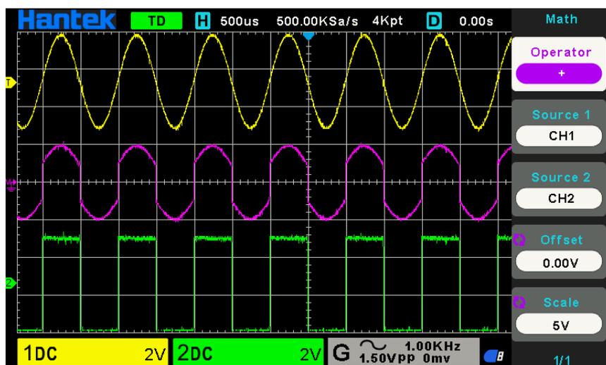
4. Press the **Scale** softkey, and turn the Multifunctional Knob to select the vertical scale.
