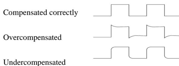
3. If necessary, use a nonmetallic screwdriver to adjust the variable capacity of your probe until the shape of the waveform turns to be the same as the above figure. Repeat this step as necessary. See the figure below for the way of adjustment.
