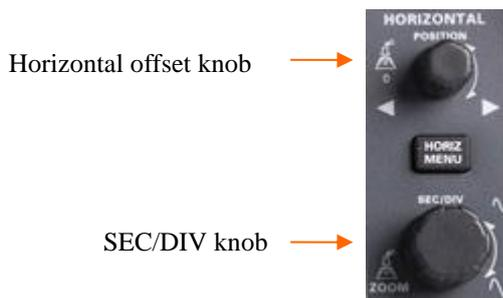
**1. Horizontal Offset Knob:** Used to control the trigger position against the screen center. Push this button to reset the trigger point back to the screen center.
