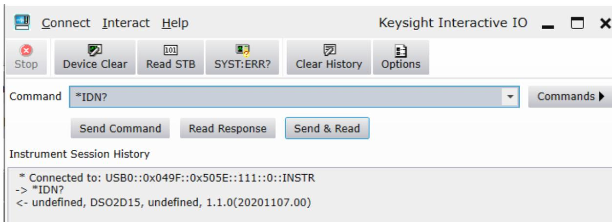
Double-click to open the host computer software, and "Connected" is displayed in the lower left corner of the interface. At this point, the host computer has been connected.
