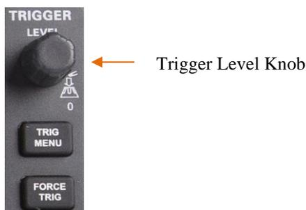
**Force Trigger:** Used to complete an acquisition regardless of an adequate trigger signal. This button becomes useless if the acquisition is already stopped.
