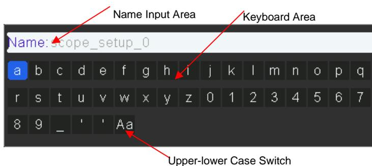
5. Turn V0 to select “Aa” and press V0 to confirm to set the input method to upper case. Turn V0 to select “DSOXXXX01” and then press V0 to input the characters successively.
