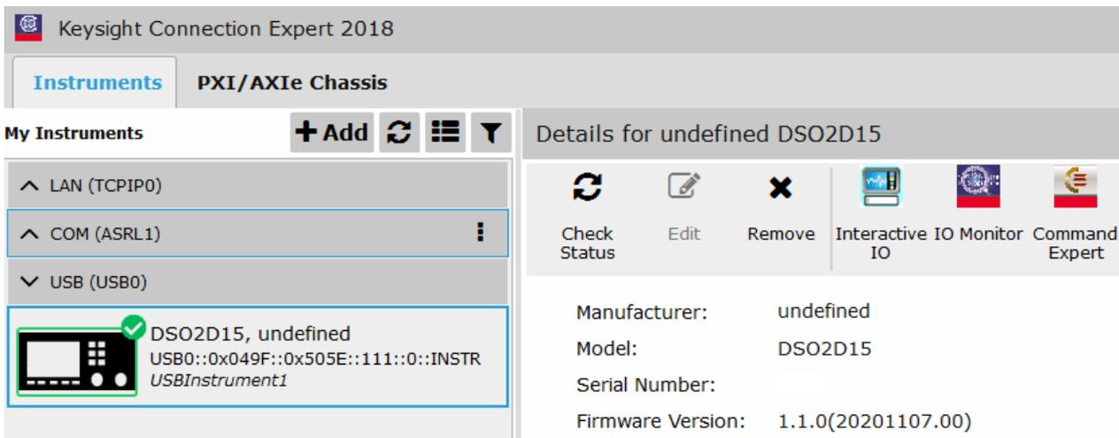
Click "Interactive IO", send an instruction arbitrarily, and the computer and the oscilloscope will communicate.
