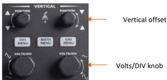
**1. Vertical Offset Knob:** Move the channel waveform up and down on the screen. In dual-window mode, move the waveform in both windows at the same time in a same direction. Push this knob to return waveform to the vertical center position on the screen. Two channels correspond to two knobs.
