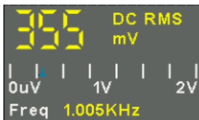
The display in the middle of the DVM box is the corresponding ratio of the current measured voltage value to the range corresponding to the eight vertical grids on the screen with the selected volt/div (turn the volt/div knob).
