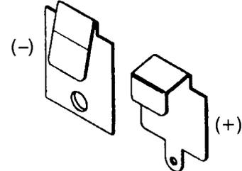
Mount the slide switch onto the foil side of the PC board. The tabs on the switch must go through the slots of the PC board. Solder the switch to the PC board.
