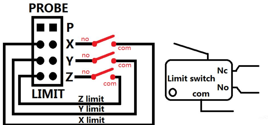
2> Input probe code: G38.2 Z-20 F3, Z axis start probe, the probe device wiring as follows:
