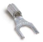
These non-insulated fork terminals are made of electrolytic copper for high conductivity. They can be installed with crimping tools having a single indentor or double indentor (recommended for solid wire). Serrated barrel increase grip on wire. Wire range identification is stamped on the tongue of each terminal.
